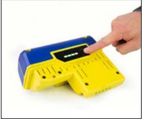
1. Each battery has been designed with a Battery Status Indicator to identify the battery charge level. To use this feature, simple press the Battery Status Button located on the battery. Four green lights indicate that the battery is fully charged.
