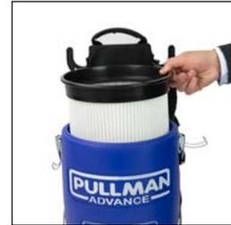
2. Next, remove the Patented Filter drum & tap gently to clean.
